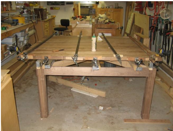
Figure 12 Final glue up of top. Note use of 7 clamps
