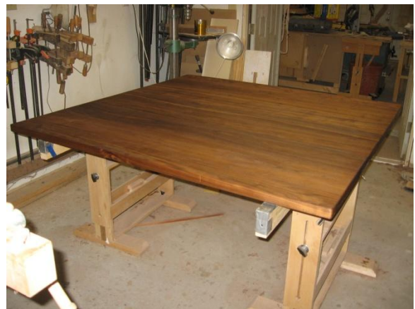
Figure 15 Table top after second round of sanding in Watco oil
