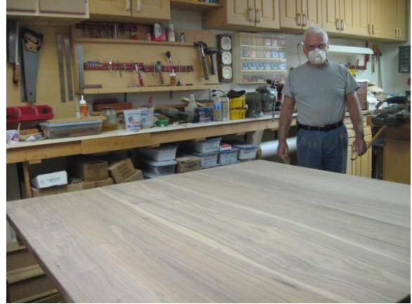
Figure 14 Sheet sanding completed.
