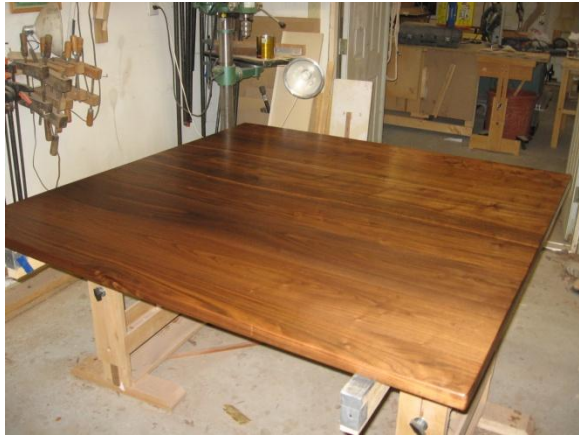
Figure 16 Table top after application of last coat of polyurethane varnish.
