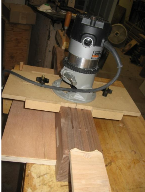
Figure 9 Fluting jig. Positioned on the leg and moved from stop block to stop block.
