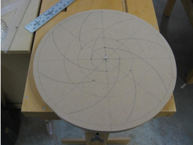
Figure 6 All 8 spirals. Note that the second half don't go all the way into the middle circle
