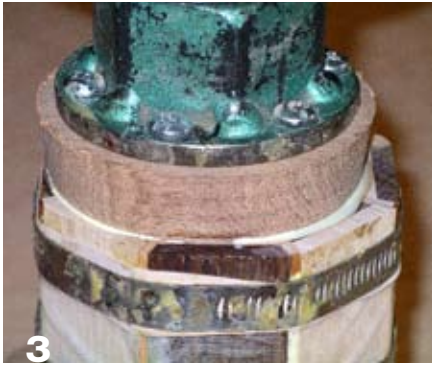
3 Pipe clamps provide the ideal pressure for gluing up the stave mug wrap.
