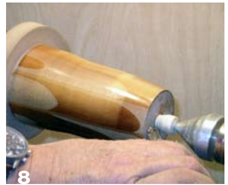
8 With the mug held between a jam chuck and a live center, use a scraper to turn the bottom.
