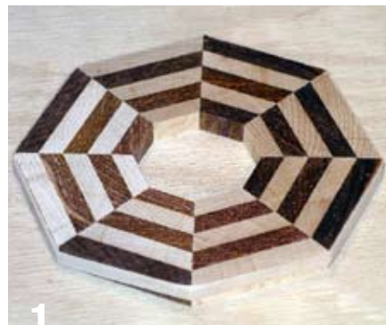
1 Cut 5 eight short pieces to test that your saw blade is set precisely at 22.5-degrees.
