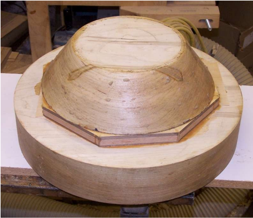
Photo #5: Blank stacked and glued
