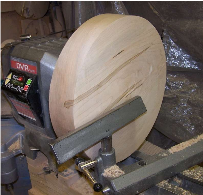
Photo 1: Blank mounted on the lathe and trued up.
