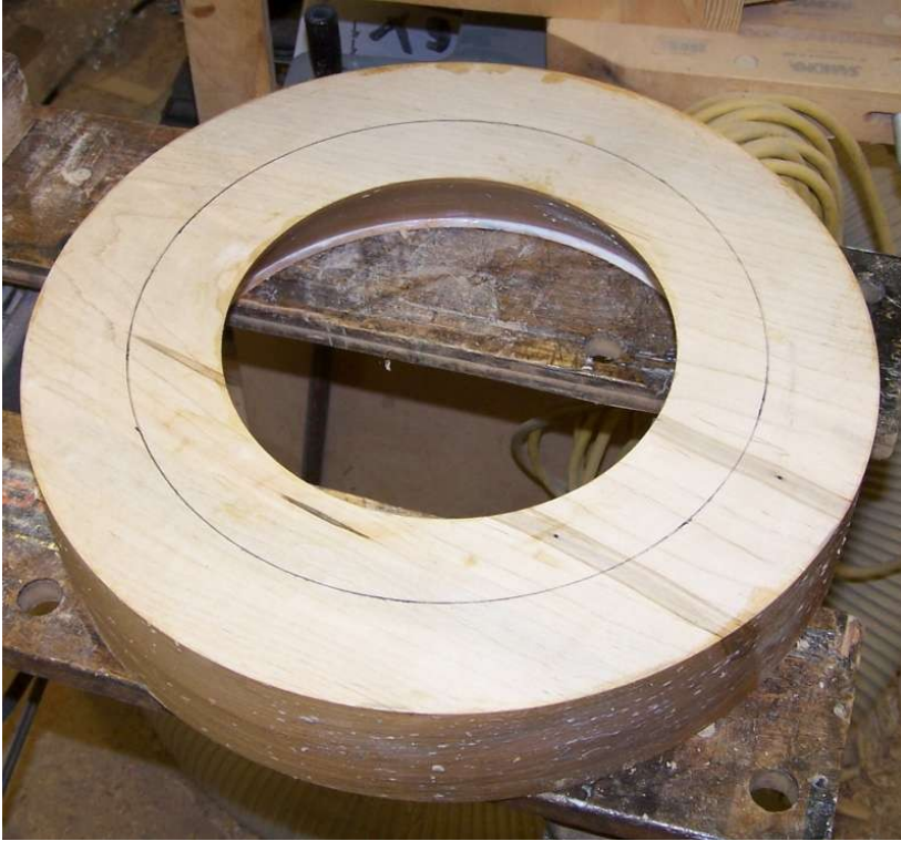
Photo #4: This shows the amount of overlap available for the glue joint.
