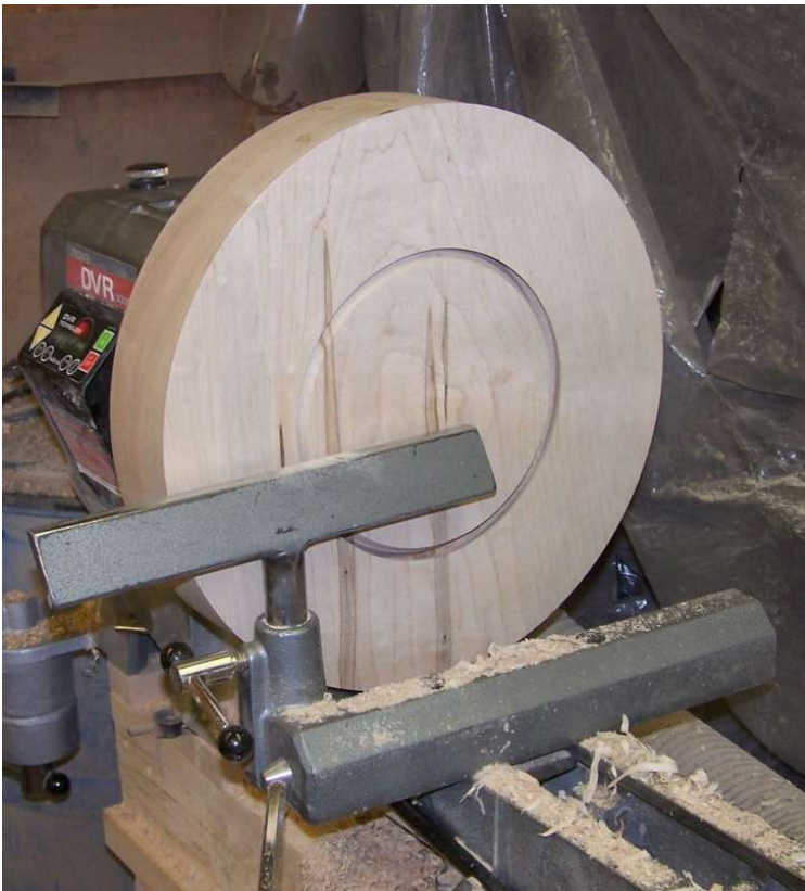
Photo #2: Parting cut
